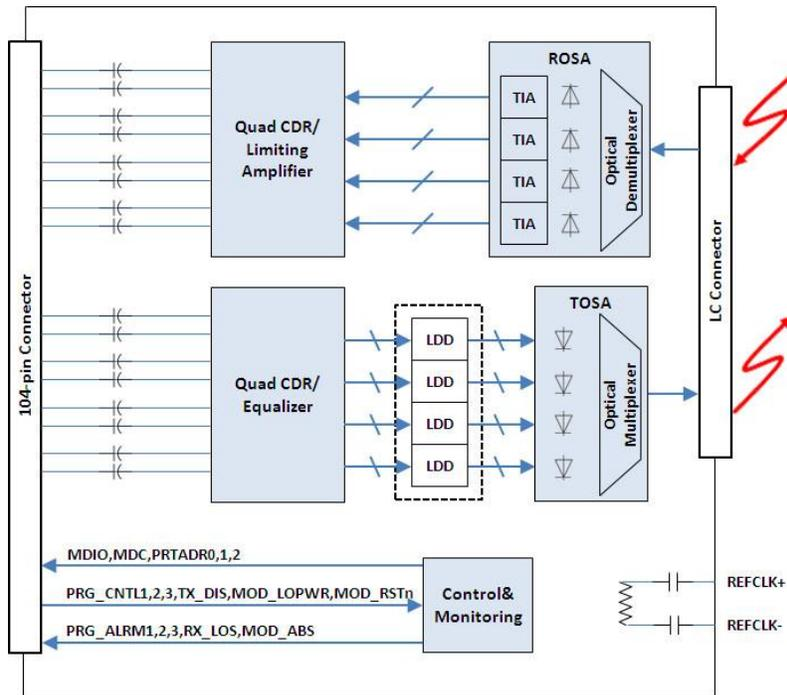
**CFP2 LR4 Optical Transceiver functional block diagram**
