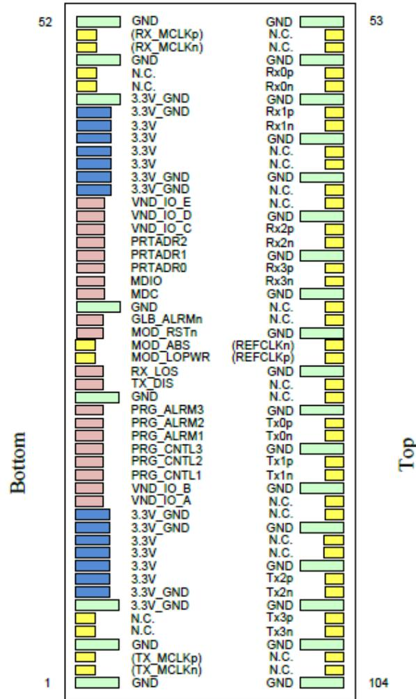
CFP2 optical transceiver pin-out
