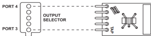
Legacy 7-DC directional coupler oriented with port 3 as the tap leg.
