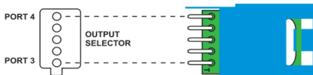
7-DC-xx-5-1000-WC directional coupler with cover has guides that only allow it to be oriented with port 3 as the tap leg. Remove the cover (blue) and rotate 180° as shown below to orient port 4 as the tap leg.
