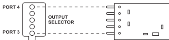
Legacy 7-DC directional coupler or 7-DC-xx-5-1000-WC with cover removed oriented with port 4 as the tap leg
