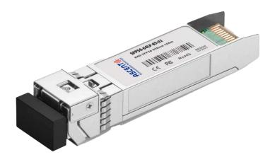
The 64GBASE-SW SFP56 Optical Transceiver Module is a high-performance solution designed for short-reach fiber communication applications. Operating over multimode fiber (MMF) at an 850 nm wavelength, it supports data rates up to 64G and link distances of up to 100 meters. With its compact SFP56 form factor and LC duplex connector, the module provides a reliable, space-efficient interface for high-speed data transmission.
